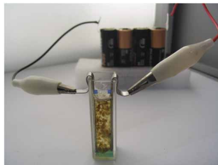
Fig. 6. A simple reaction set-up for electro-polymerization of CHCl 3 .
